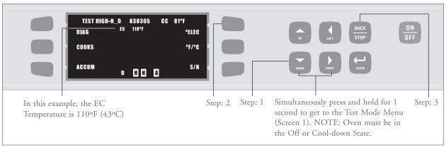
FIGURE 36: Viewing the Electrical Compartment (EC) Temperature
